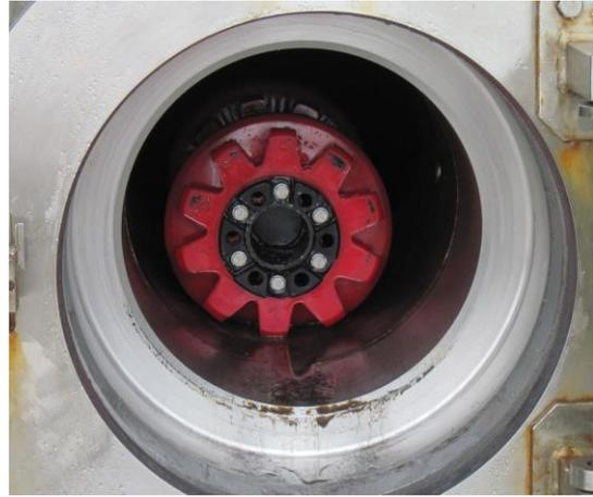
**Figure 6: Brush pig in receiver during pre-ILI cleaning**
