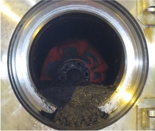
**Figure 5: De-sanding pig and debris in receiver during pre-ILI cleaning**
