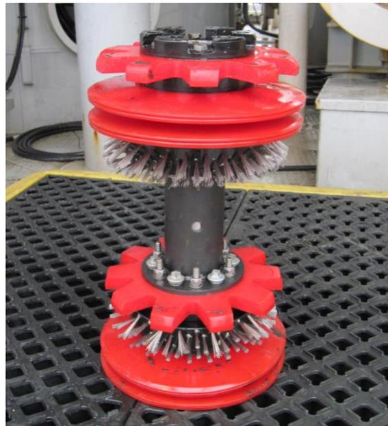
**Figure 7: Brush pig with brushes permanently deformed backwards after passage through multi-diameter pipeline**
