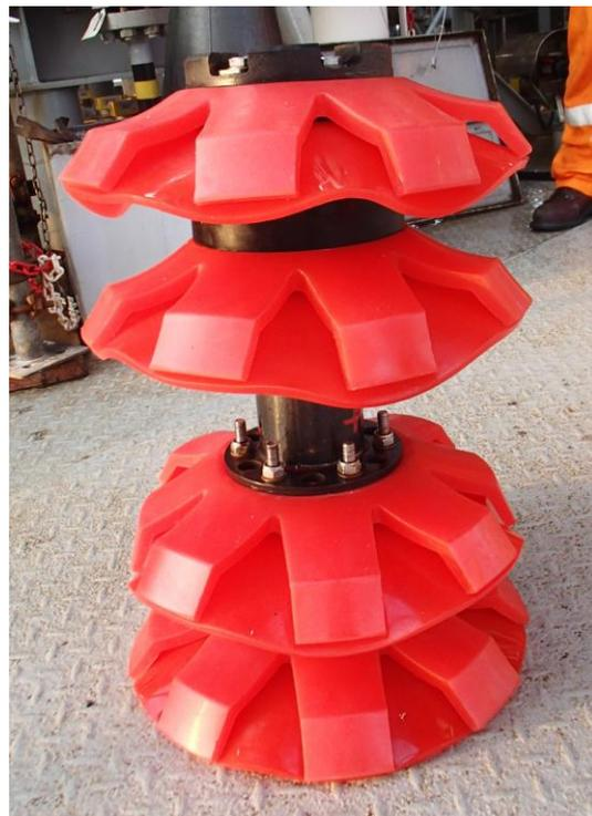
Figure 2: De-sanding pig
